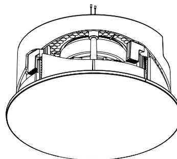
**6** Align the grille to the speaker and firmly attach the grille to the speaker.
