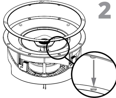
**2** Position the rubber ring on the speaker so that the 8 rubber grommets align to the 8 holes of the speaker; press firmly to connect the ring to the speaker.
