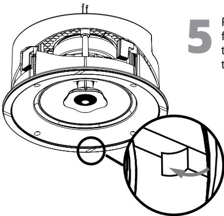
**5** Remove the backing from the 4 pieces of tape that are attached to the rubber ring.
