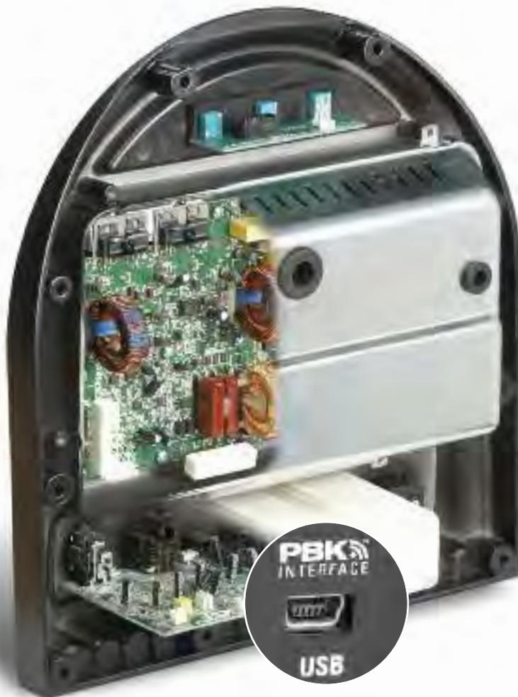
State-of-the-art Ultra-Class-D™ amplifier housed inside the gorgeous industrial design cabinet. Form following function is once again the guiding principle ...
