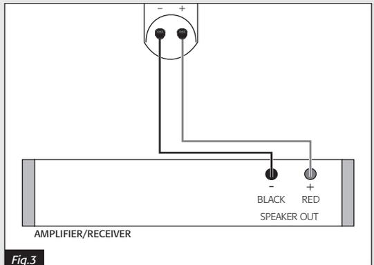
Connect the red (+) amplifier terminal to the red (+) speaker terminal and the black (-) to the black (-). Tighten the posts firmly by hand, but don't over-tighten them.
