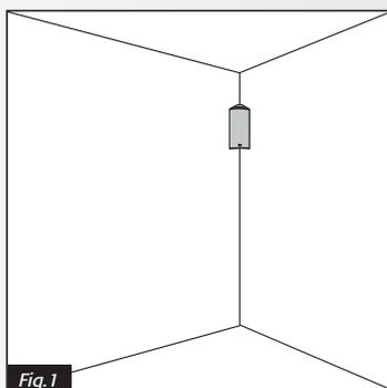
Cinema™ speakers also have holes, spaced 60mm apart, in the backs of their enclosures which fit a variety of Premier™ mounting brackets (*fig.1*) (*optional extra - see dealer for more information*). If wall-mounting, take extra care in installation - we always recommend the use of safety straps as secondary restraints.
